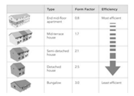
An increase in the Surface to Volume ratio of 10% (the building in the middle below) would require 20mm of insulation more than the good form on the left to achieve the same level of insulation. The one on the right (a 20% higher S/V ratio) would require an extra 40mm of insulation. Therefore compactness should be encouraged.
